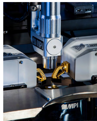
Fig. 3: The waveguide probes directly mounted at the output of the mm-wave VNA converters. Picture is courtesy of Rohde & Schwarz.
